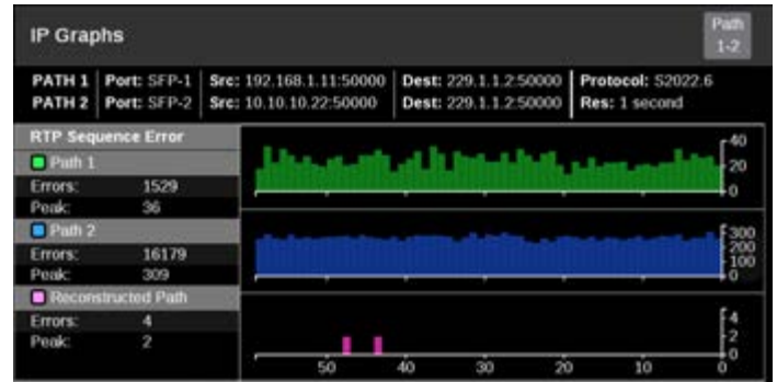
RTP Sequence Error incident graph for monitoring the errors detected over time
