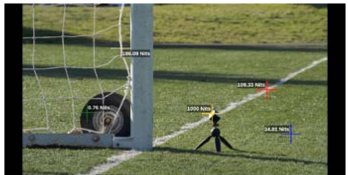
Light meter reads the luminance level of the targeted objects.
